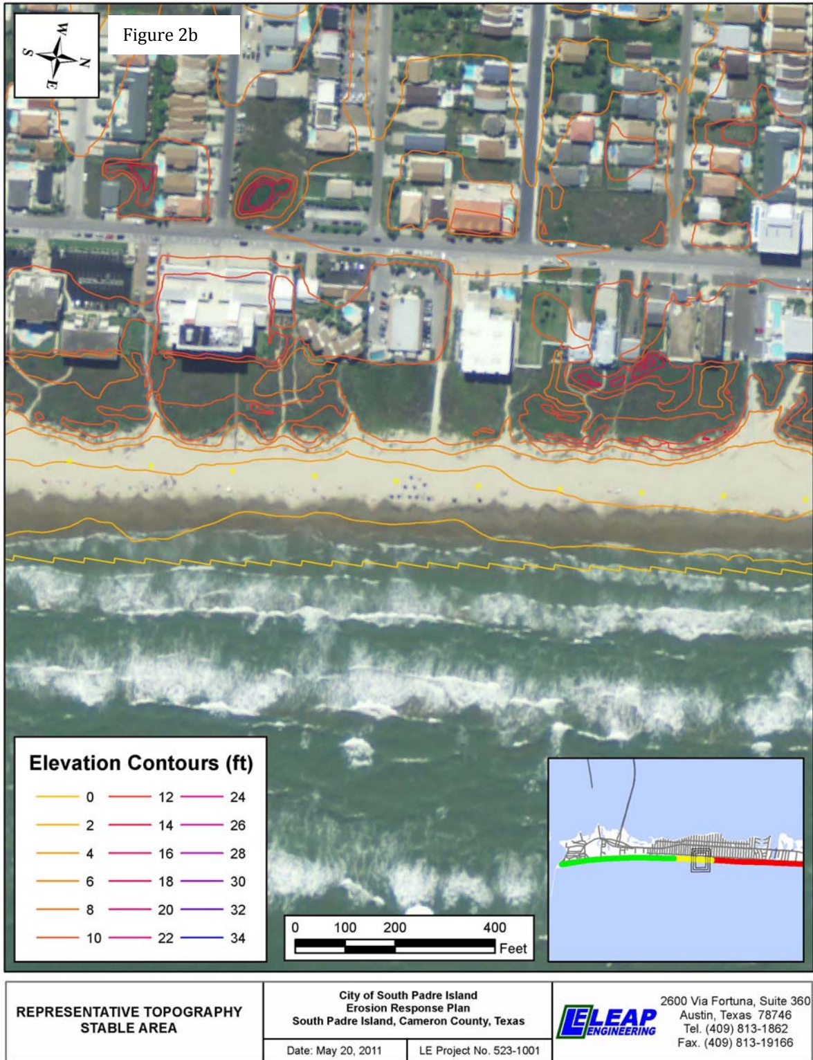
Figure 2b depicts a typical section of the beach/dune system in the stable area. Here, dunes are typically narrower than those found further south and dune
