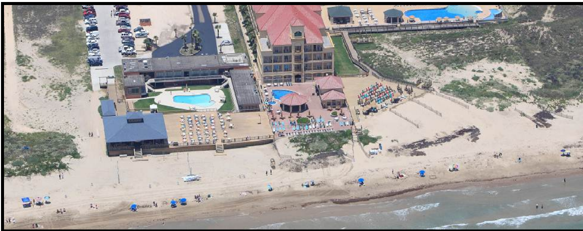
Photo 2 - Dunes are limited or poorly formed in eroding areas along the northern reach of the City's beach. (Photograph by Richard Stockton, May 2012)
