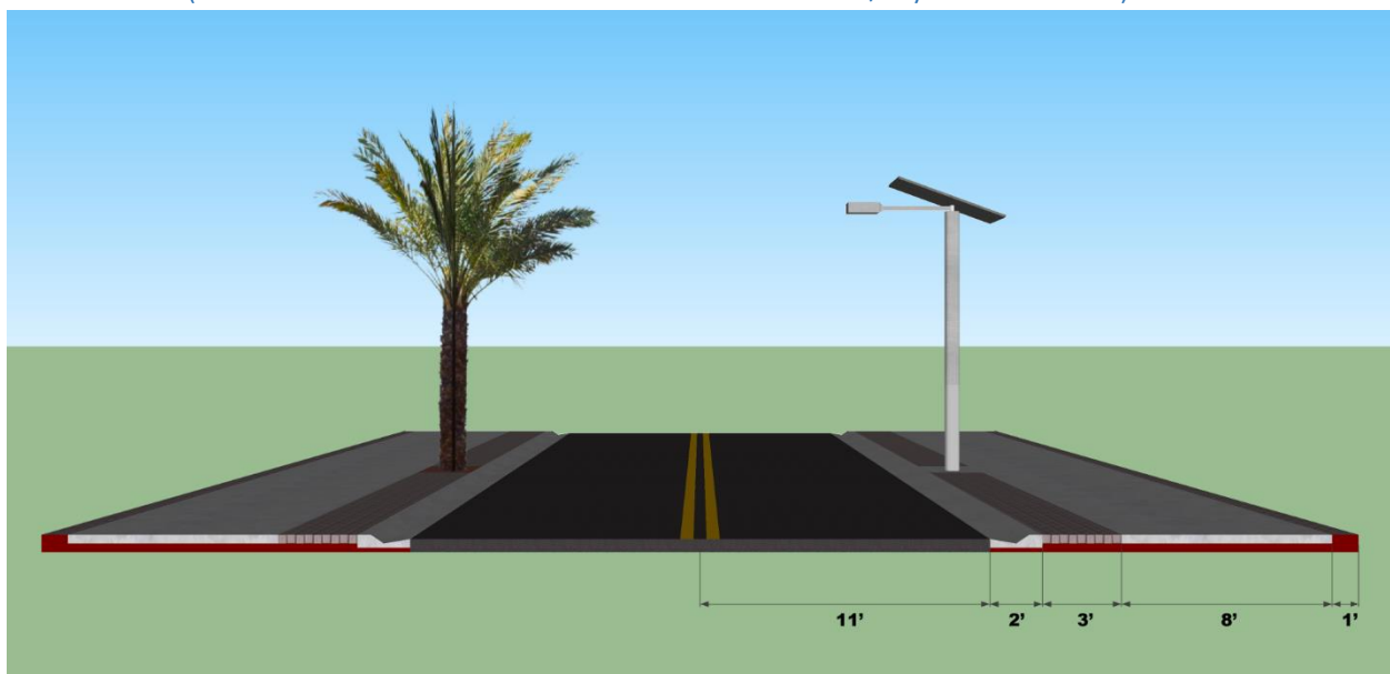
Alternative (vehicle-accessible sidewalk with mountable/lay-down curbs)
