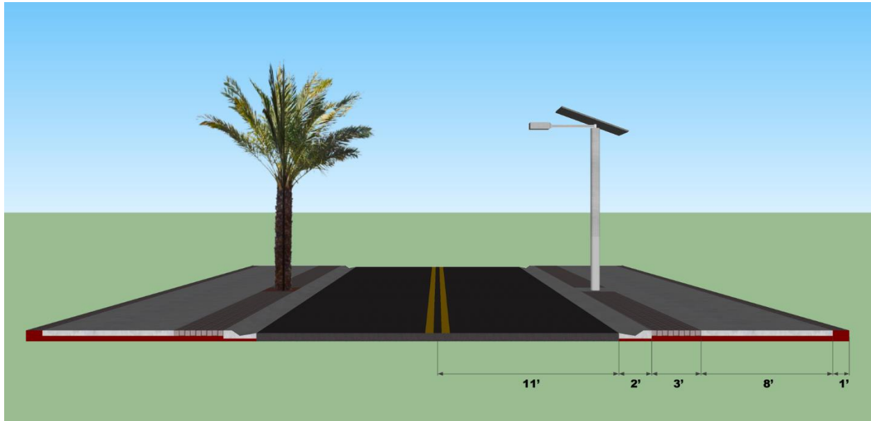
Alternative (vehicle-accessible sidewalk with mountable/lay-down curbs)
